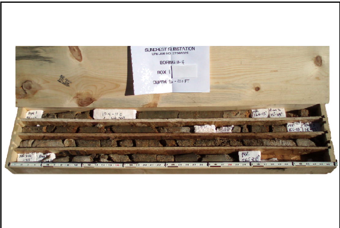
Boring B-04, Depth Interval 9.6 to 28.0 feet
